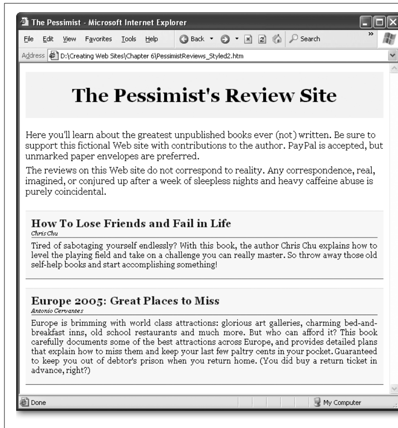
Figure 6-17: In this example, each review is wrapped in a <div> tag. The <div> tag applies a background color and some borders, separating the reviews from the rest of the page. Techniques like these can help organize dense pages with lots of information.
